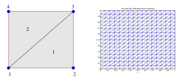
Figure 29: (left) The initial discretisation of a rectangle (right) and the obtained discretisation after four refinement steps.
