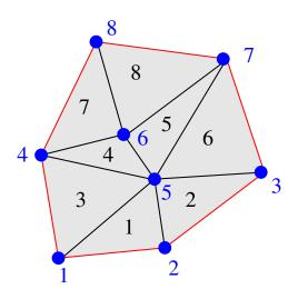
Figure 33: A triangular finite element mesh
