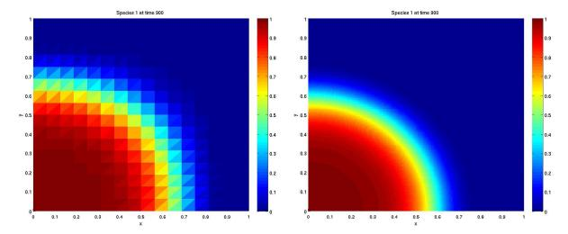
Figure 32: (left) The solution u(t, x) at time t = 900 if the domain has been discretised three time (512 elements) and (right) the solution u(t, x) at times t = 900 if the domain has been discretised five times (32768 elements)
